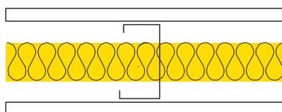
70mm Metal Stud Wall with 25mm APR 1200
